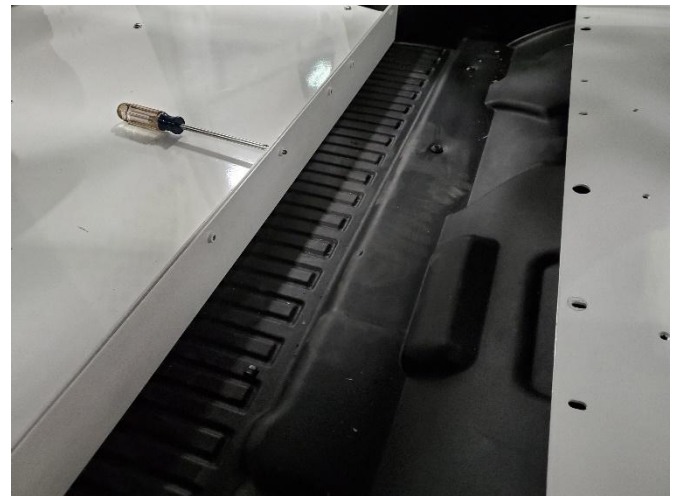
Attach plate to fill gap below floor using (3) 1/4" x 3/4" Phillips head bolts and flat washers.
