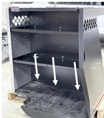
Once everything is tight, secure bottom of divider to K9 floor using four (4) 1/4" x 3/4" self-threading screws.
