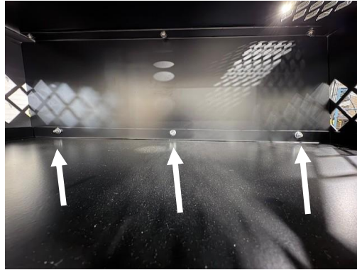
Loosely attach top shelf (56193/56194) to divider using three (3) 1/4" x 1/2" carriage bolts (inserted from K9 side) and serrated nuts.
