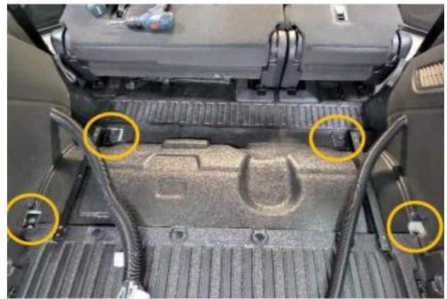
Determine 3rd row seat bolt locations in floor and loosely attach front floor brackets (24810) with supplied M10 bolts (16518). Temporarily remove OEM M12 bolts from the rear seat belt anchor locations. (T50 Torx)
