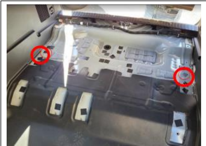
For a vehicle with no 3 rd row seat, remove tape over two circled holes and tap with M12 x 1.75 thread.
