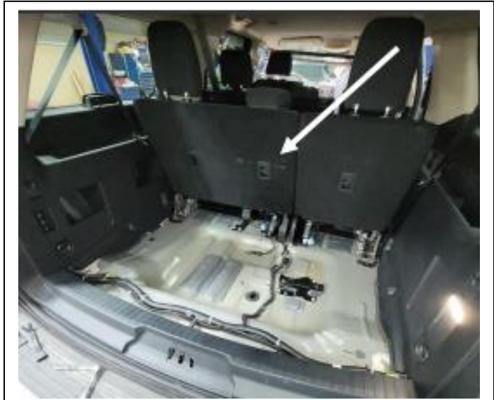
Remove 3 rd row seats if applicable. Note: Tape over unused seat mount holes in floor.
