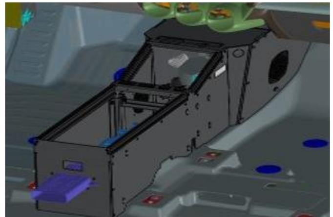
In console delete model cut ducting to size.
