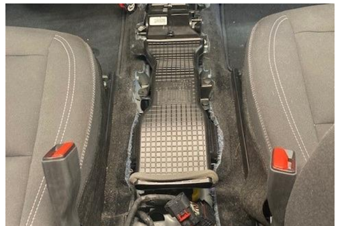
After all bolts (8 in total) are removed and wire harnesses are disconnected, carefully remove OEM console
