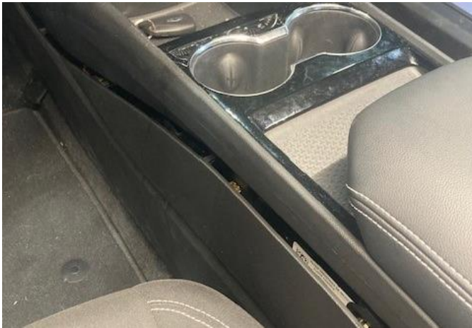
Fully remove side trim panel from OEM console – Repeat on passenger side
