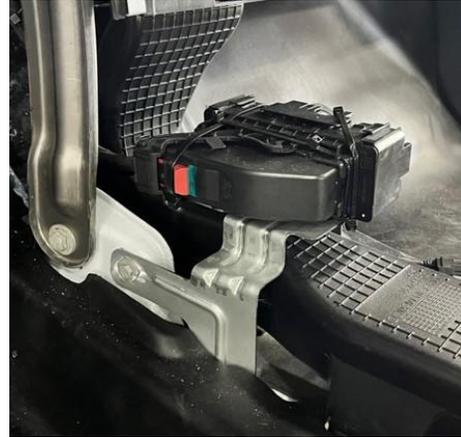
In console delete model remove fuse block from OEM bracket – after removal, use Havis brackets and remount
