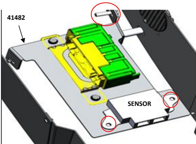
Use OEM bolt to mount wire harness bracket (41842)
