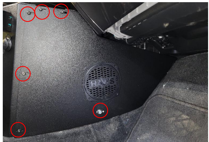
Install trim plates using torx screws and insert M6 x 65mm screw thru M6 split lock washer, then thru M6 flat washer, then thru side panel, then thru 1.5" long Nylon spacer
