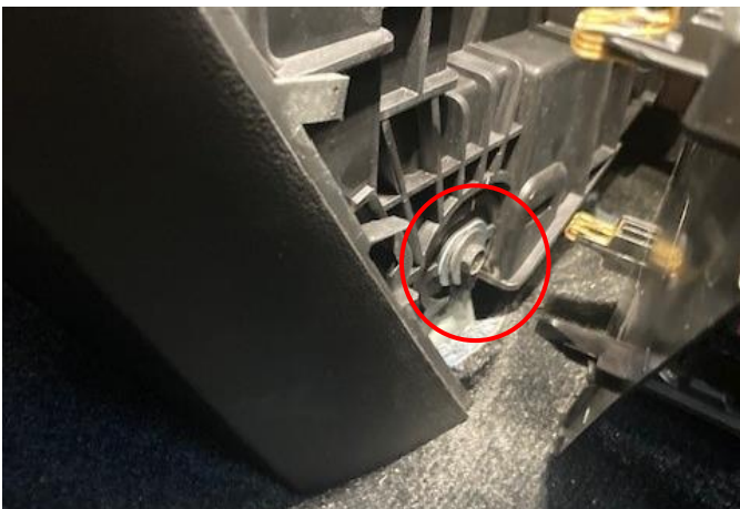
Remove OEM hardware at rear of center console – repeat on both sides
