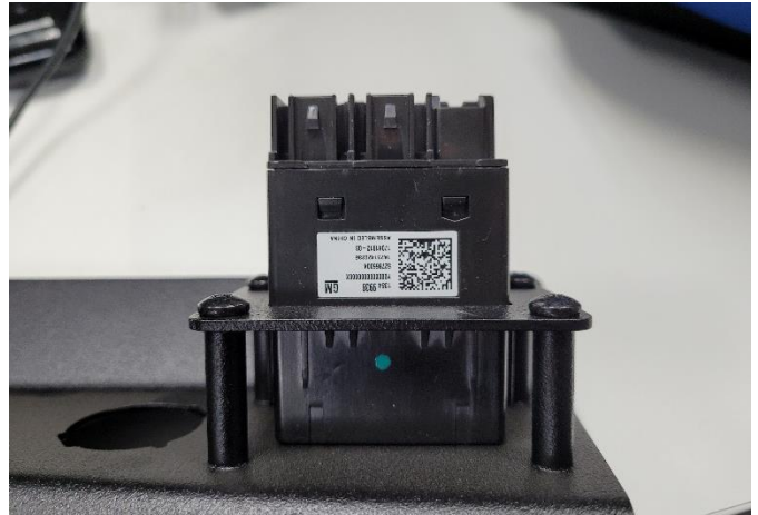
In console version relocate OEM USB using (38475) and (4) (16399) #10-32 x1/2 PH screws
