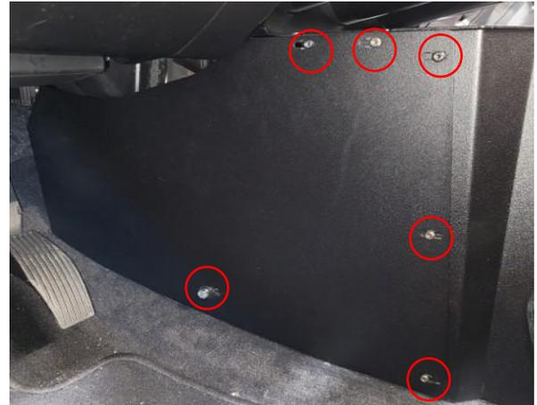
Install DS trim plate using torx screws and insert M6 x 65mm screw thru M6 split lock washer, then thru M6 flat washer, then thru side panel, then thru 1.125" long **Aluminum** spacer
