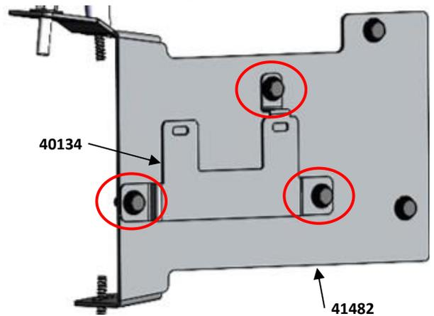
Attach fuse block bracket (40134) to wire harness bracket (41842) using ¼-20x3/4 screws, flat washer, and flange nuts
