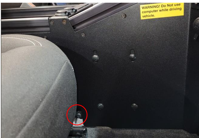
Attach front mounting bracket to GM studs using two OEM screws – repeat both sides
