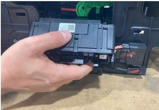
Models with OEM console remove fuse block and remount using Havis brackets (40134) and (41842)
