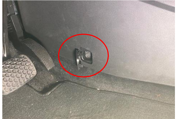
Start by removing OEM console - Keep and reuse OEM hardware after removal
