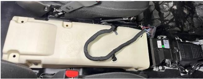
In 'console delete' version remove plastic tunnel mount cover – keep and reuse hardware
