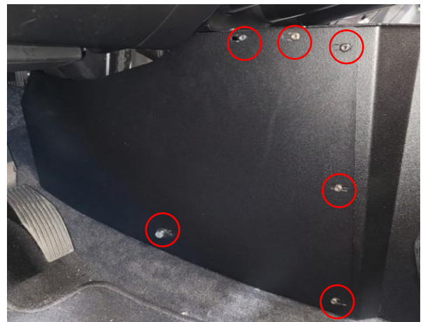
Install DS trim plate using torx screws and insert M6 x 65mm screw thru M6 split lock washer, then thru M6 flat washer, then thru side panel, then thru 1.125" long Aluminum spacer
