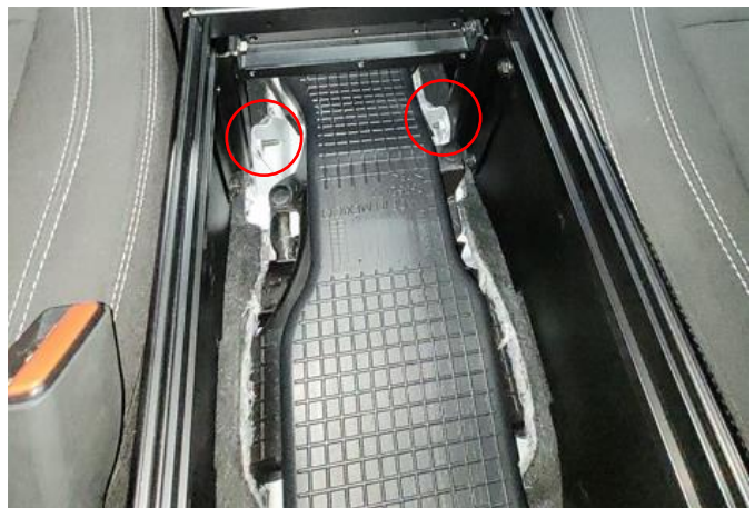
Attach front mounting bracket to GM studs using two OEM screws – see next picture for placement
