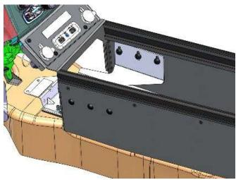
Loosely attach main housing to front mounting bracket using carriage bolt and serrated nuts provided.
