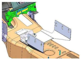
Attach lower mounting bracket from console to OEM studs. Ignition key sense module bracket goes over the supplied bracket. Loosely tighten using previously removed OEM nuts.
