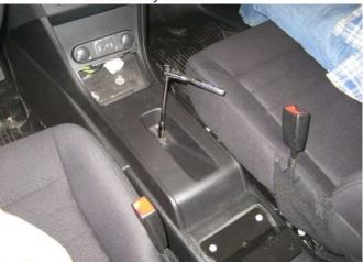
Remove bolts that hold underside of extrusion to rear floor bracket. Remove rear floor bracket bolts and center console bolt. (10mm).
