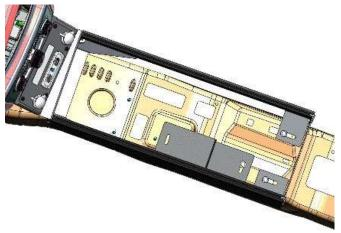
Cover (11209) is provided to guard the OEM sensor on the transmission hump. Attach cover using  $\frac{1}{4}$  x  $\frac{3}{4}$ " self-threading screw.
