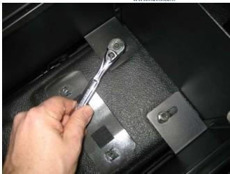
Use  $\frac{1}{4}$  x  $\frac{3}{4}$ " self-threading screws to loosely attach the rear of the console to existing floor inserts. Inserts located under rubber floor mat as shown.
