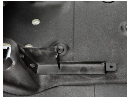
Using OEM bolts from the storage cubby, install mounting brackets (40621) on DS and PS. **NOTE: Mounting Bracket is the same for both sides. Orientation from the PS is as shown above.**
