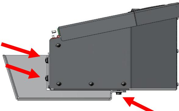
Install Carriage Bolts (16222) and 1/4-20 Nuts (16013) from inside the storage box into the Mounting Bracket (40621) in 3 positions shown. Repeat for other side. Tighten all fasteners.
