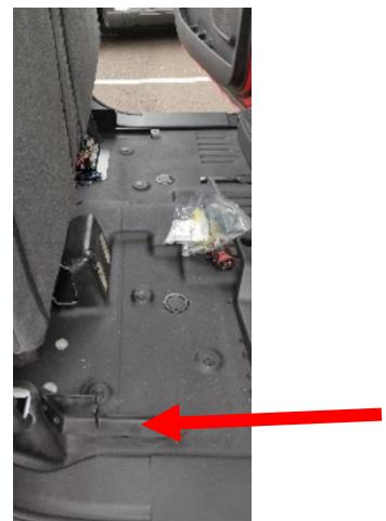
Place storage box on top of Mounting Brackets (40621) and loosely install M6 bolts (41586) into center mounting holes
