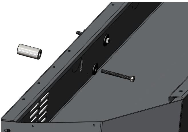
Insert M6 bolt (41586), Washer (16127) and AL Spacer (41587) into slotted holes of storage box.
