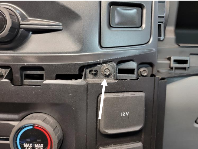
Remove OEM 7mm head fastener from above 12v socket.
