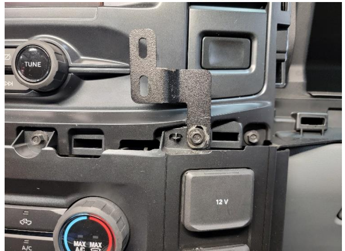
Install lower mounting tab using 7mm fastener.
