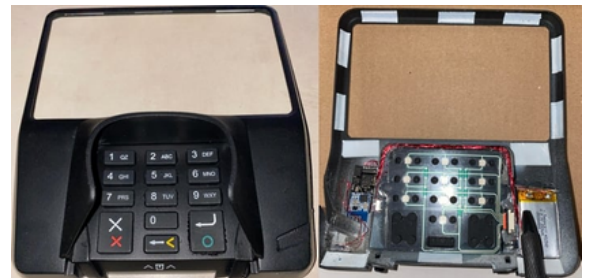
Pictured: Card skimmer removed from payment device
