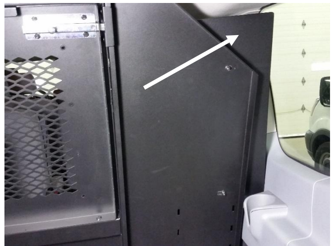
Attach upper and lower side filler panels with 1/4" x 3/4" carriage bolts and nuts. Tighten all hardware.
