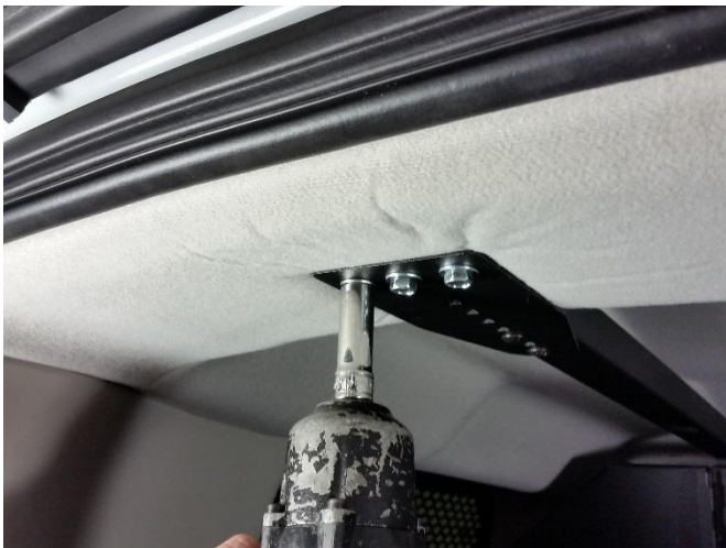
Attach upper mounting bracket to rear door header frame with 1/4" x 1" lag bolts.
