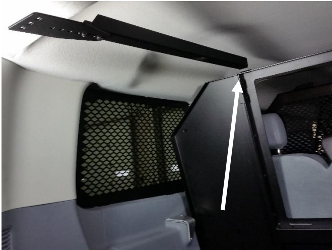
Attach upper mounting bracket to top of partition frame with 1/4" x 3/4" carriage bolts and nuts
