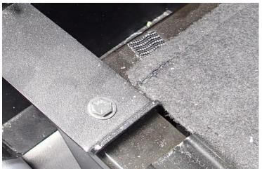
Attach lower support brackets (CM007238) to predrilled holes in seat base using 1/4"x 3/4" hex bolts, 1/4" washers, and nuts. (one on each side)
