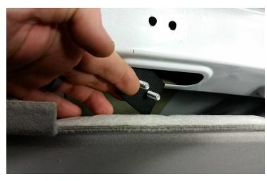
Place stud plate (CM003457) into holes up through the large opening in the rib with the studs facing rearward.
