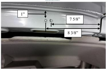
Mark and drill two (2) holes as shown with a 9/32" drill bit. Both holes measure 1" down from the top of the rib. Measure across from cross support seam 7 5/8" and 8 3/8".
