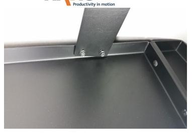
Attach partition to upper roof brackets using two (2) 1/4" x 3/4" carriage bolts and serrated nuts.
