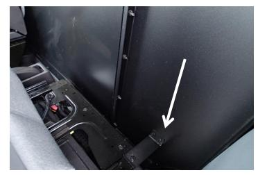
Slide partition in through the side door and prop into position. Attach to the lower support brackets using two (2) 1/4"x 3/4" carriage bolts and 1/4" nuts. P-MFK-13\_INST\_5-25
