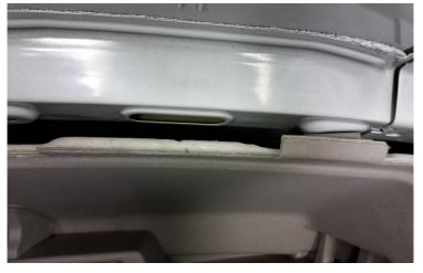
Remove middle section of headliner to expose the cross support rib over the front seats.
