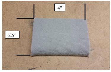
Remove the headliner and cut a section for bracket clearance approximately 4" x 2.5". Repeat for both sides. Reinstall headliner.
