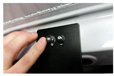
Attach Upper roof bracket to stud plate using two (2) 1/4" serrated nuts (GSM30023)
