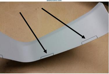
Draw a line between the points to help with maintaining a straight cut. Remove (notch) plastic from the panel as needed for mounting tab clearance.
