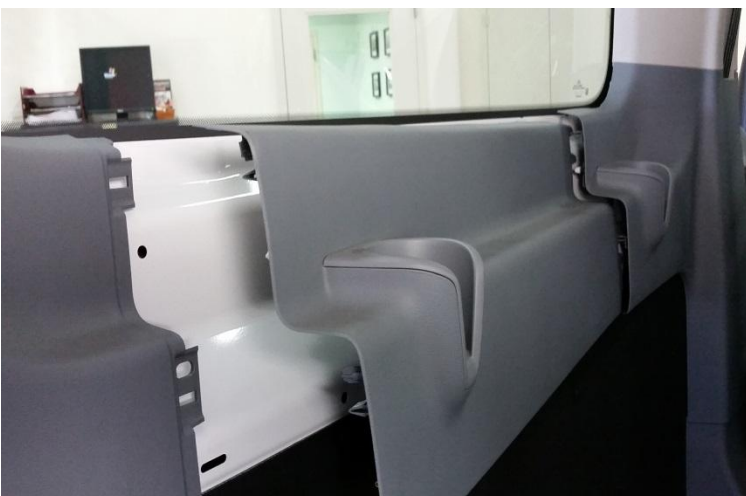
Carefully remove the vans interior panels including the door panels.
