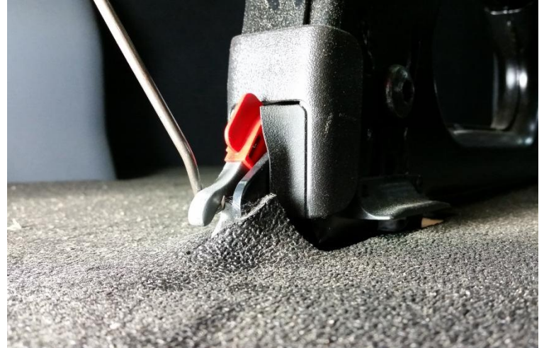
When the latch is hooked, simply pull up to release the latch.
