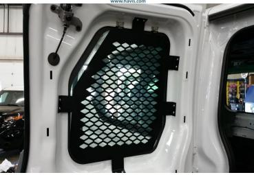
Attach screen to door using #10 x 1/2" screws (GSM33194)
