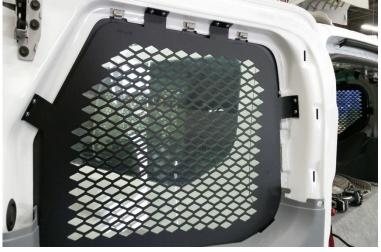
When all guards are hung, begin to loosely place the trim panels back on the van. Mark the trim on either side of the mounting tabs for notching.
