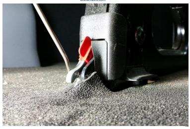
When the latch is hooked, simply pull up to release the latch.
