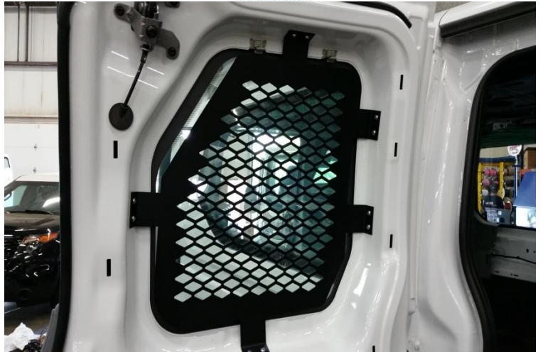
Attach screen to door using #10 x 1/2" screws (GSM33194)
