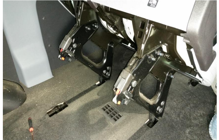
When both latches are released push the seat forward to remove. The front is hooked and will need to be slid rearwards.
