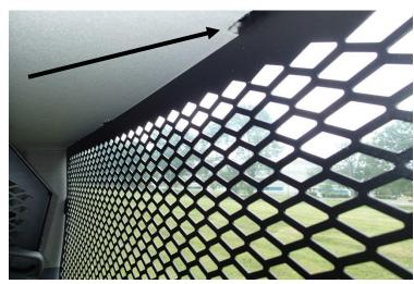
The headliner will need to notch around the tabs so that it sits properly above the screens.
