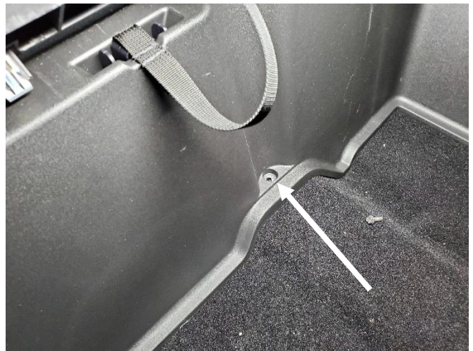
Locate and remove (2) Phillips head screws from forward storage area. (1 each side)
