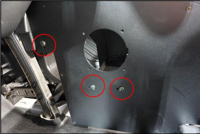
Once aligned use (3) carriage bolts (16222) and nuts (16013) to attach console to middle bracket (39444) and front bracket (39445)
