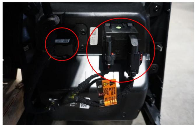
Disconnect USB and 12V socket from OEM console
