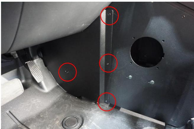
Install trim panel (39452) to the driver side. 3 screws (16425) will attach to the console and 1 will mount to OEM slot (see previous picture)
