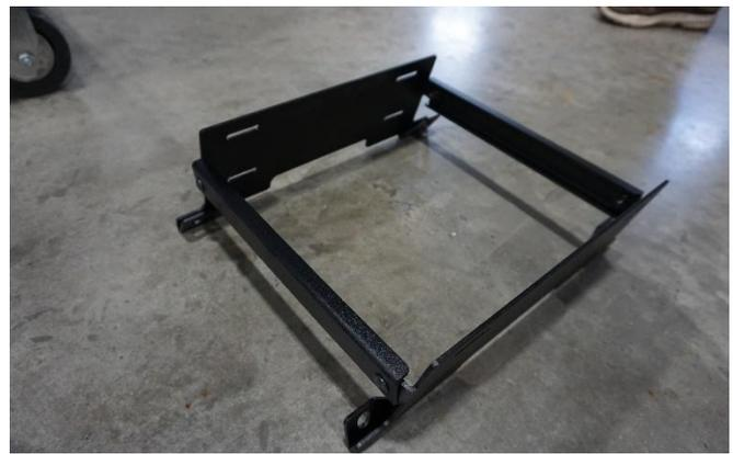
Loosely assemble rear mounting brackets (2) (39443) and (2) (39446) using carriage bolts (16222) and serrated nuts (16013)
