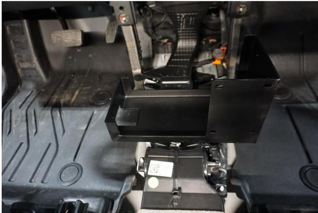
Position tunnel/middle bracket (39444) in place
