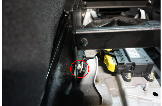
Use previously removed (4 total) OEM bolts to mount brackets – Then go back and tighten bracket hardware (16222 and 16013)
