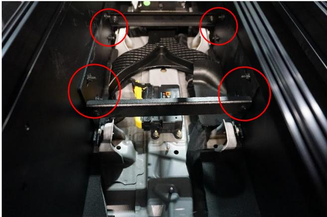
Attach console to previously installed rear mounting brackets using (8) carriage bolts (16222) and (8) nuts (16013)
