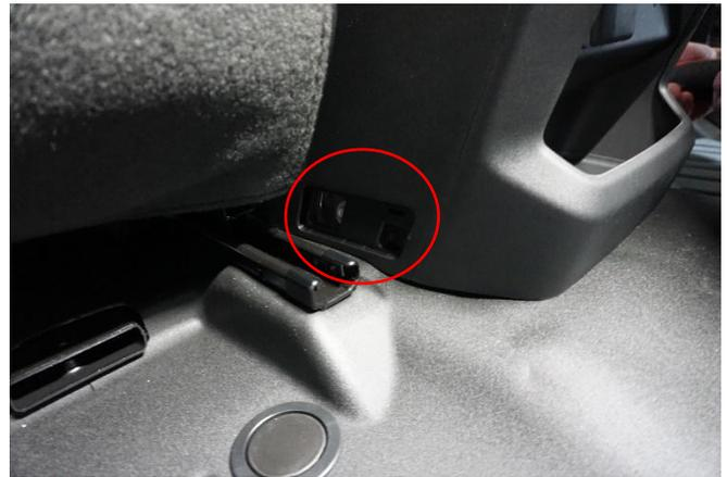
Remove rear console bolts – Repeat for passenger side of console
