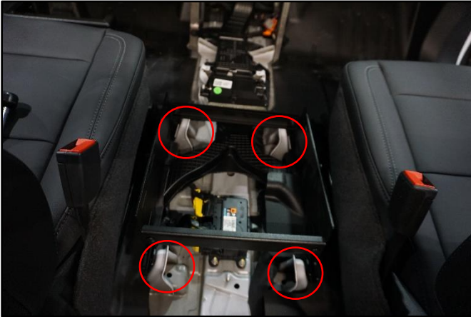
Fit loosely assembled mounting brackets over OEM mounting points circled in red
