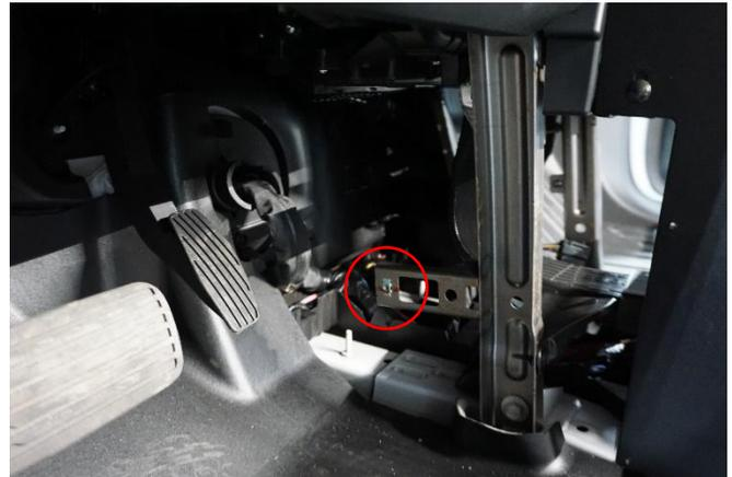
Install trim panel (39452) to the driver side. 3 screws will attach to the console and 1 will mount
