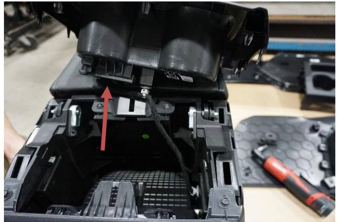
Remove Key Sensor from under OEM rear cup holder
