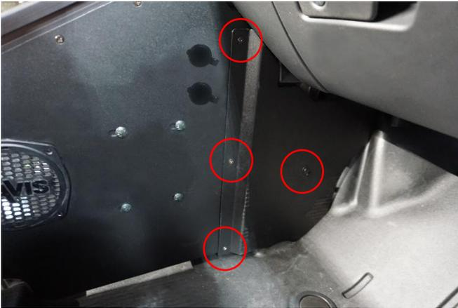
Install trim panel (39453) to the passenger side. (3) screws (16425) will attach to the console and (1) will mount to OEM slot (see previous picture)
