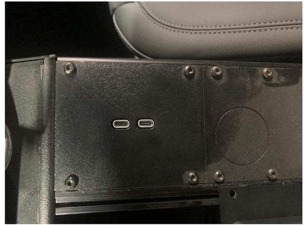
Relocate previously removed USB to the 3.3" wide section using plate 39454, bracket 38475, and (4) 16399 screws
