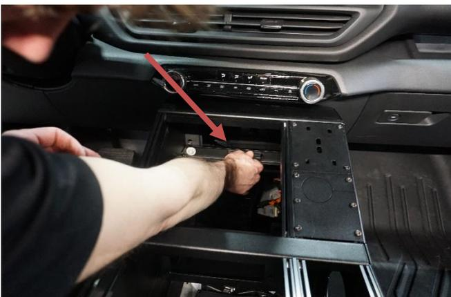
Relocate key sensor to front mounting bracket (39445)
