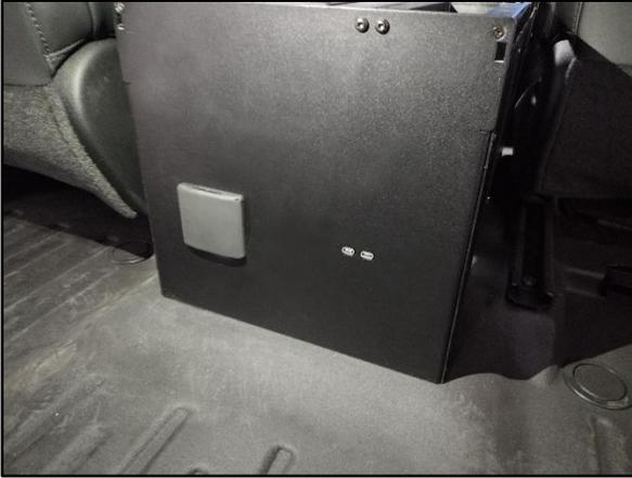
Relocate 12V socket and USB module to rear of console. Use bracket 38475 and (4) 16399 screws to relocate USB
