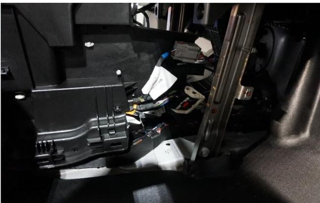
Disconnect wire harnesses under dash before removing OEM console completely
