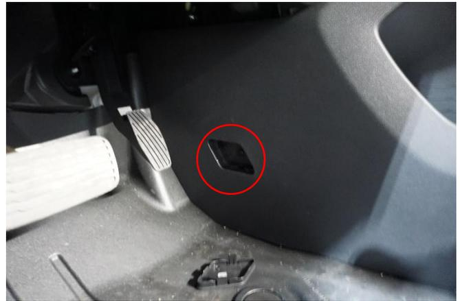
Start by removing side panels and bolt (10 mm) from OEM console - Repeat for passenger side
