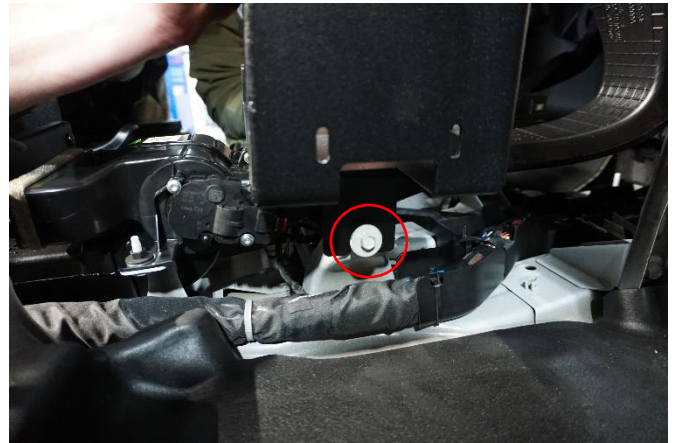
Use previously removed OEM bolts and loosely attach bracket (39444)
