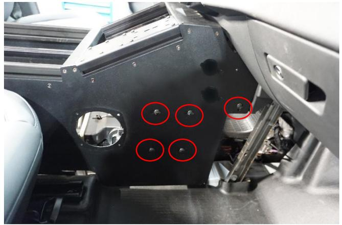
Repeat on passenger side with 5 carriage bolts (16222) and nuts (16013)
