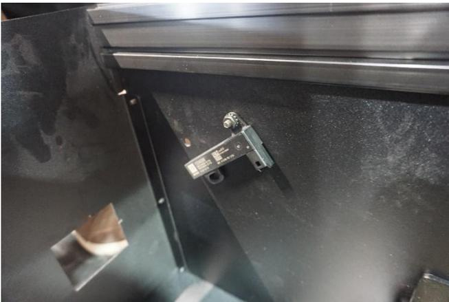
Relocated OEM Key Sensor to the rear driver side panel using (2) (16399) and (16017)
