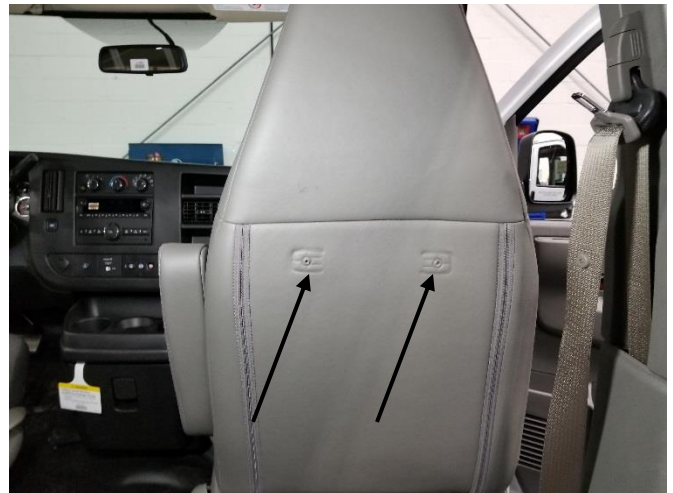
Remove the grab handle from the rear of the seat.
