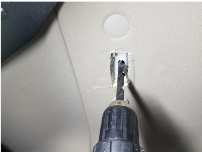
Drill three (3) 25/64" holes in cross member. Drill small pilot holes first to insure proper positioning.
