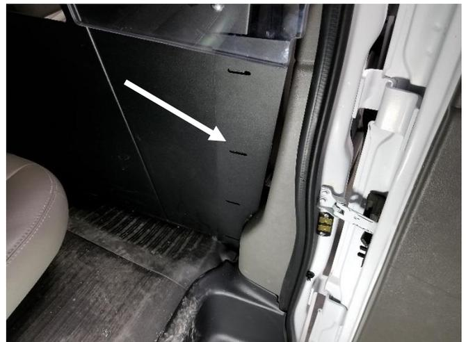
Place lower filler in van and line up to slots in the partition wing.
