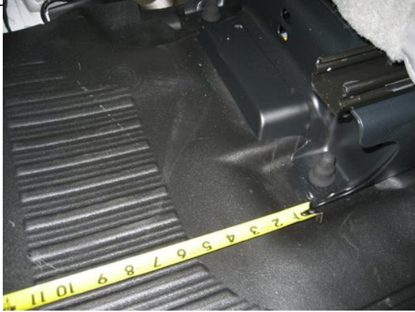
Driver Side partition mounting area.
