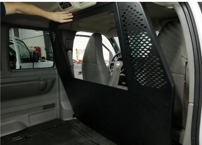
Attach upper trim panel to top of partition with 1/4" x 3/4" carriage bolts and serrated nuts. (nuts on top)
