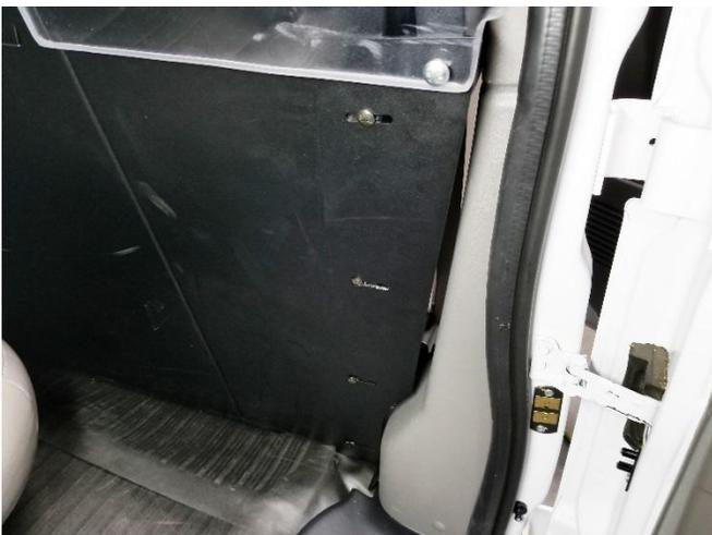
Attach lower filler panel using 1/4" x 3/4" carriage bolts and serrated nuts.
