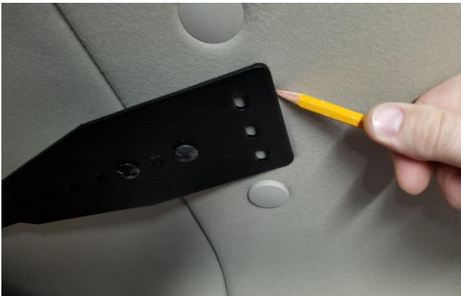
Trace outline of bracket onto headliner with pencil. Note: C-MFK-8 uses 1/4" x 1" self-threading screws instead of Rivnuts. Next 3 steps not necessary for P-FRONT-2 / P-MFK-8 application.
