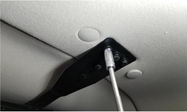
Attach partition mounting brackets using 1/4" x 3/4" hex head bolts, lock and flat washers.
