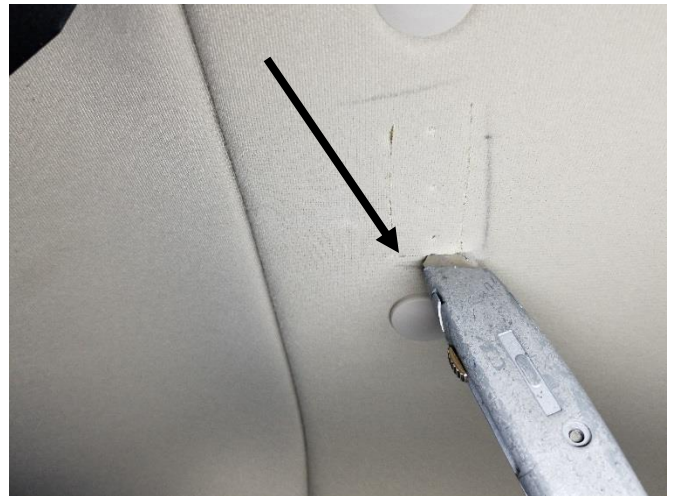
Move bracket out of the way and cut headliner around the previously marked three (3) holes. Be sure to stay on the inside of the penciled outline.
