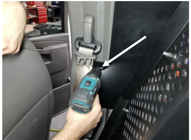
Drill 1/8" pilot holes in the "B" pillar after confirming you are clear of all OEM wiring
