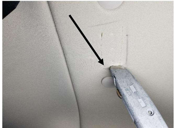
Move bracket out of the way and cut headliner around the previously marked three (3) holes.
