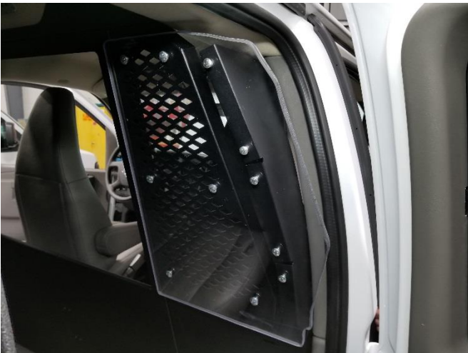
Drill 1/4" holes in Lexan and attach filler using carriage bolts, washers, and nylon stop nuts.
