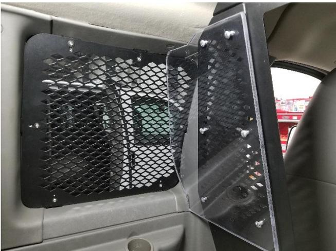
Attach upper filler panels using 1/4" x 3/4" carriage bolts, washers, and nylon stop nuts.
