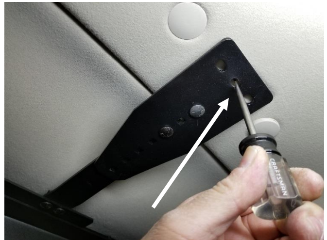
Push partition forward so that the bracket falls in line with the factory push pins in the headliner. Mark location for three (3) mounting holes in the headliner and metal cross member.
