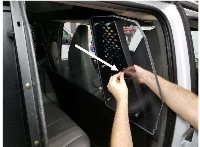
Place Lexan upper filler on partition and line up to door and window. Mark and drill 1/4" holes in Lexan to match holes in partition wing.
