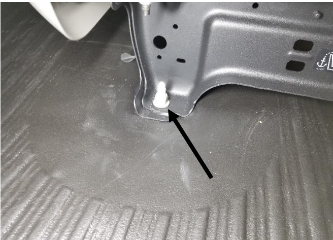
Remove the nuts from the rear inner seat studs. (18mm socket) Do not remove nuts for P-MFK-8 application. See next page for P-MFK-8 floor mount details.
