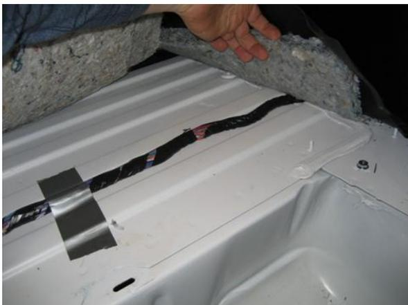
Passenger side harness repositioned in between floor ribs. Cutting harness wrap in order to lay wire more flat is suggested to minimize chance of partition pinching wires.
