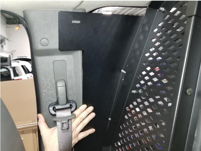
Place passenger side upper metal filler panel onto "B" pillar and Lexan filler.
