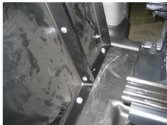
Carefully Drill and lag bolt to the vehicle floor. Mounting upper brackets is the same for both P-FRONT-1 / P-MFK-4 and P-FRONT-2 / P-MFK-8
