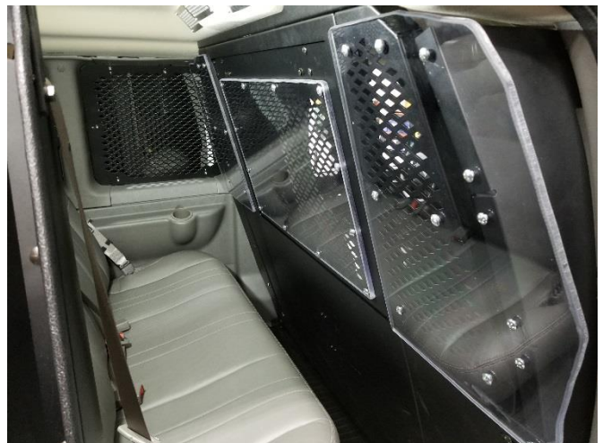
Installation is now complete. Make sure emergency hatch removes properly.
