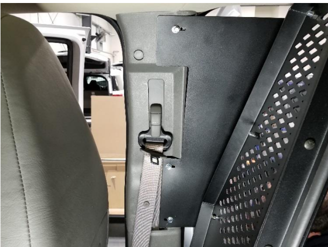
Attach metal filler to "B" pillar using Three (3) 1/4" x 1.5" lag bolts.
