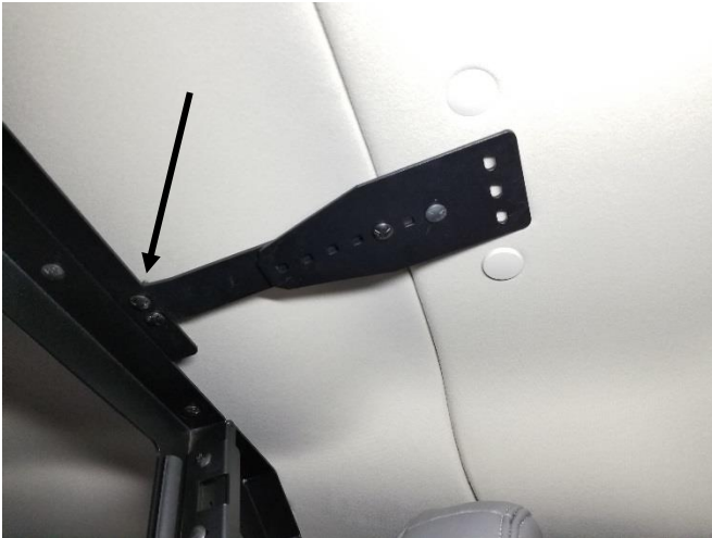
Loosely attach upper mounting bracket assembly to top flange of partition using 1/4" x 3/4" carriage bolts and nuts.
