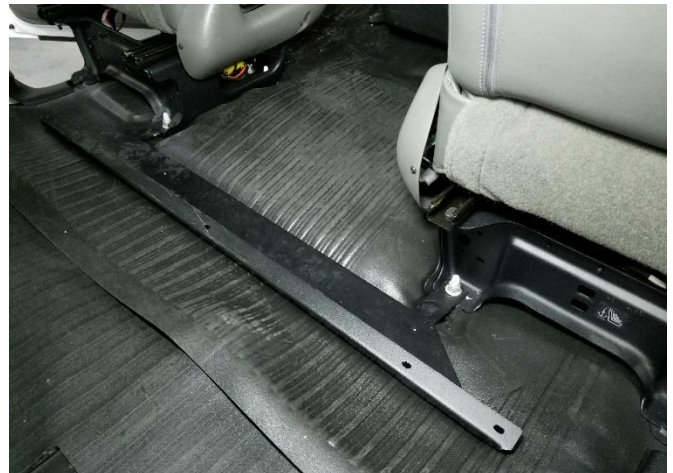
Place the lower mounting bracket onto the seat studs, replace OEM nuts and tighten. Bracket not used in P-MFK-8 application.
