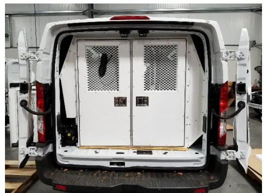
Install the rear door frame assembly into the van and line up to benches.
