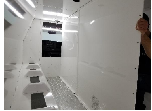
Place middle divider section into van and line up bolt holes to front divider section.
