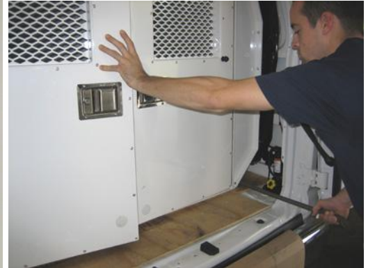
Check measurements in PT-A-3XX instructions. Center the insert in the van and line up to the measurements.
