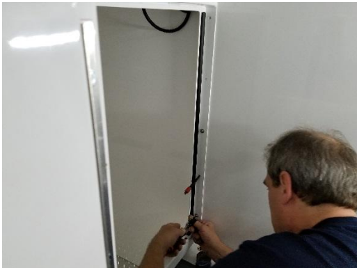
Use alignment tool to help line up middle bulkhead and both dividers. Bolt the panels together using 1/4" x 3/4" stainless socket button head bolt and washer.
