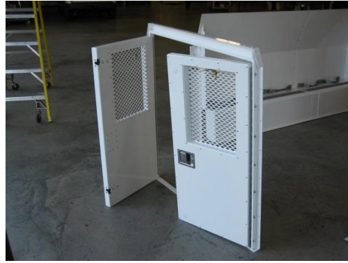
Rear bulkhead/door assembly
