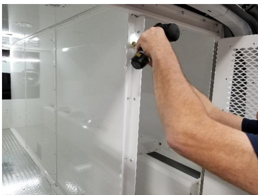
Attach divider to door frame using #10 x 1/2" flat head machine screws and nylock nuts. Place weather stripping over bolts.
