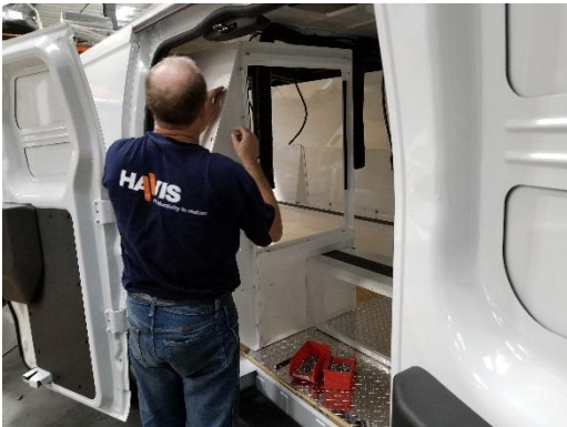
Attach the bench and wall to the bulkhead using 1/4" x 3/4" carriage bolts and serrated nuts.
