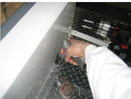
Drill a 3/16" hole through the diamond plate and bench lip only. Do not drill through OEM van floor.
