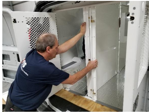
Place the rear divider section into the van and line up to middle divider and door frame.
