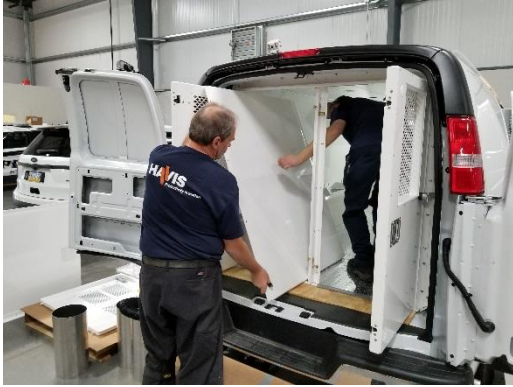
With the help of a second installer. Lift the front divider wall section into the van.
