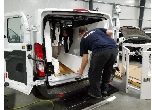
Install the passenger side rear bench and wall assembly into the van and line up half bulkhead.
