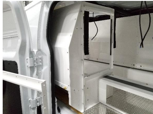
Roughly square up kit and line up to van side door opening.
