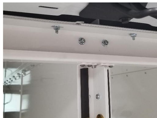
Install two (2) 1/4" x 3/4" carriage bolts and serrated nuts at the top of rear divider to bulkhead frame.
