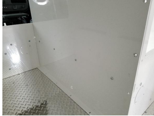
Line up to the front bulkhead and third row bench. Bolt to front bulkhead and bench using 1/4" x 3/4" carriage bolts and serrated nuts.
