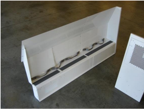
Driver Side full length Bench/Wall assembly with Front bulkhead wing section.
