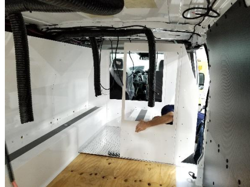
Attach to the third compartment bench using 1/4" x 3/4" carriage bolts and serrated nuts.
