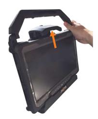
3. Once unlatched grab both sides of tablet, rock the top forward and carefully lift out of Docking Station, top end first.
