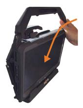
3. While pivoting the tablet, apply downward pressure to align with the Docking Station's Locator Bar. Depress the Latch Handle to secure tablet in place. You will hear an audible click when Latch Hook is fully engaged.
