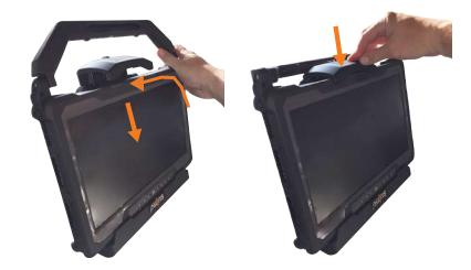
4. For theft deterrence, secure tablet by locking Docking Station with supplied key (Hardware Kit Item 2).
