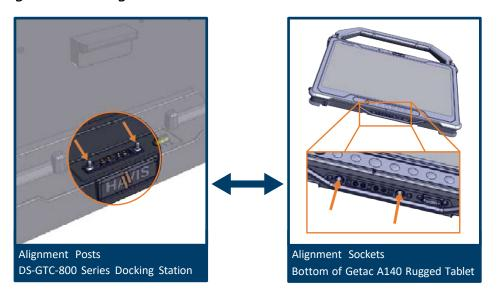
Docking Station must be unlatched before docking your tablet. Push down on the Barrel Lock button and release slowly. Without a tablet present you may have to lift up lightly on the front of the Latch Hook to fully release.
