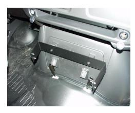
Attach vehicle-mounting bracket using OEM hardware
