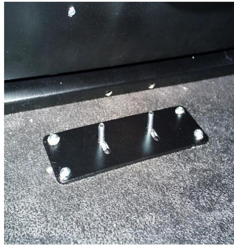
Position console and mark location of floor mounting plate. Drill 1/8" pilot holes and attach using #10 x 1" sheet metal screws.
