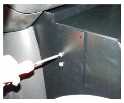
Loosely attach console and side fillers to vehicle mounting bracket using ½" x ¾" Phillips bolts and washers
