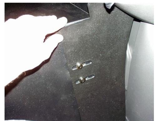
Adjust side fillers to contour with OEM molding.
