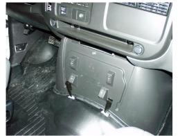
Remove (4) 10mm bolts from inside lower OEM console pocket
