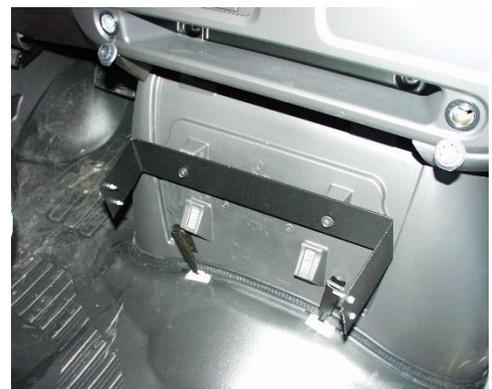
Attach vehicle-mounting bracket using OEM hardware
