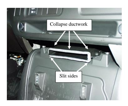
It is recommended to collapse the plastic ductwork to prevent air from blowing into the console. This will force air out the other vents.
