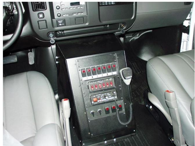
Attach console to vehicle mount brackets.
