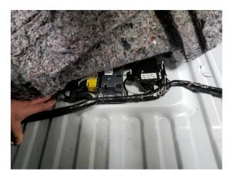
The cover will need to be removed from the sensors between the seats. Move the OEM harness to the rear of the sensors and loosely secure in place.
