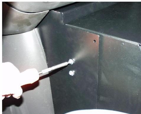
Loosely attach console and side fillers to vehicle mounting bracket using 1/4" x 3/4" Phillips bolts and washers.
