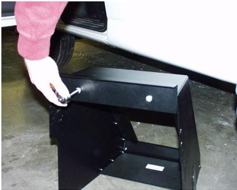
Attach upper filler panel using 1/4" x 3/4" Phillips bolts, washers and serrated nuts
