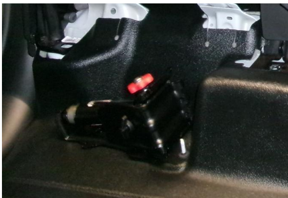
Remove the jack and relocate where appropriate.
