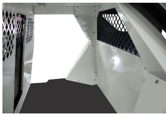
Place rubber mat into insert when silicone is dry. Installation is now complete.
