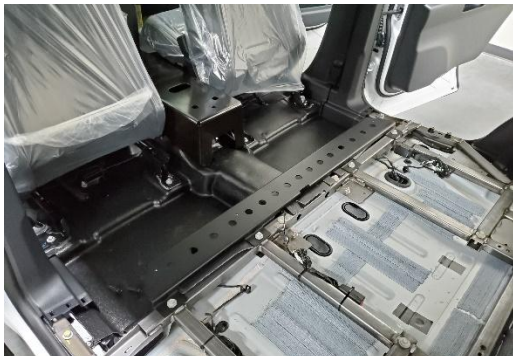
Use OEM bolts to attach K9 kit front floor bracket to OEM seat mount locations.
