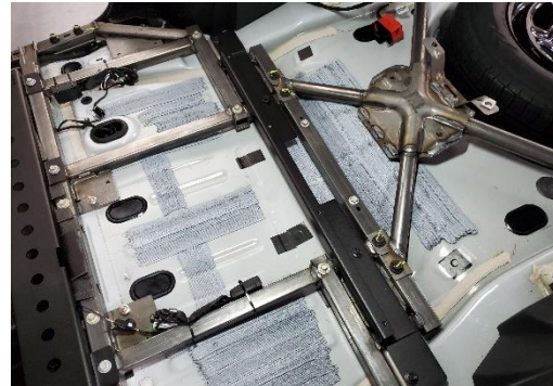
Use OEM bolts to attach K9 kit rear floor bracket to OEM cross brace.
