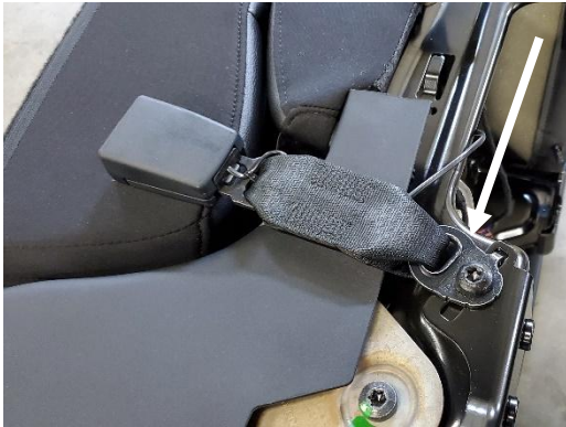
The (3) seat belts on the back seats have built in sensors that will turn on an indicator on the dash. They must be removed from the OEM seats. (T-50 Torx)
