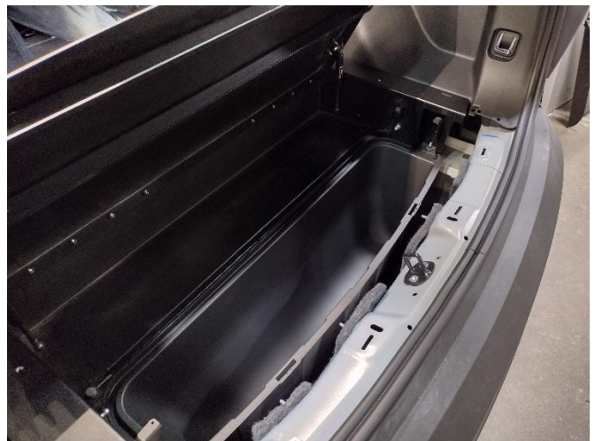
Reuse OEM mounting nuts and tighten down Place rear cover bracket behind hinge up tray and tighten with provided hardware
